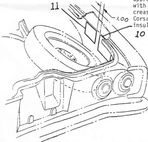
Jacking sheet-Locate at approx center of panel with top edge even with crease line. On Monza & Corsa, cement to the insulation.
